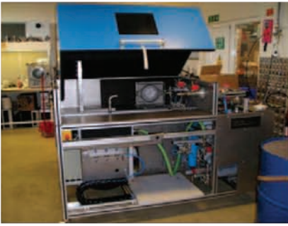
Parker Hannifin UK Ltd. has developed a custom-built test rig that generates aerosol as measured on an engine.
